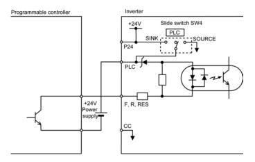
Sink (Negative) logic / Source (Positive) logic input Sink logic/source logic (input terminal logic) switching is possible.
