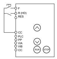
Selecting HD (operation holding) with the input terminal selection parameter
