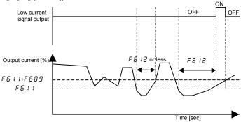
\* When setting F & I C to I (Trip), trip after low current detection time setting of F & I Z. After tripping, the low current signal remains ON.
