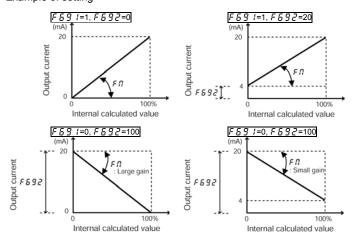
★ The analog output inclination can be adjusted using the parameter F \(\Pi\).
