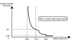
To protect the inverter, overload trip or overcurrent trip activate in a short period of time when output current reaches 110% or higher.
