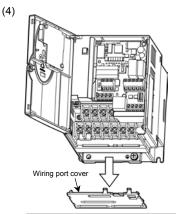
Remove the wiring port cover by pulling it down, pass cables through the wiring port, and connect the cables to the terminal board.
