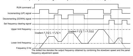
Note: If the operation frequency is set to the lower limit frequency, it will increase from 0Hz when power is turned on for the first time after the setting, and therefore the output frequency will not rise until the operation frequency reaches the lower limit frequency. (Operation at the lower limit frequency) In this case, the time required for the operation frequency to reach the lower limit frequency can be shortened by setting  $\mathcal{F}[\mathcal{E}]$  to the lower limit frequency.
