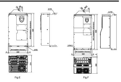
Note 1: To make it easier to grasp the dimensions of each inverter, dimensions common to all inverters in these figures are shown with numeric values but not with symbols.
