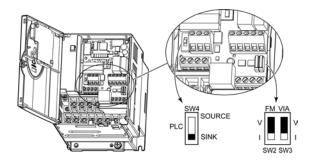
Factory default settings of slide switches SW4 : SINK (Negative) side (WN type) SOURCE (Positive) side (WP type) FM (SW2): V side
