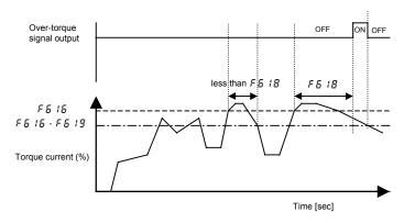
When F S I S = I (tripping), the inverter will trip if over-torque lasts for the period of time set with F S I S. In such a case, the over-torque signal remains ON.
