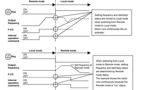
To prevent from moving the setting frequency and start/stop status of Remote mode to Local mode, the  $\mathcal{F} \supseteq \mathcal{G} S$  is set to " $\mathcal{G}$ "(Disabled). In this case,  $\binom{\widehat{CO}}{\operatorname{REM}}$  key is effective only while stopping.
