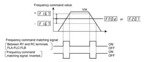
Note: This function can be used, for example, to send out a signal indicating whether the amount of processing and the amount of feedback agree with each other when the PID function is in use.
