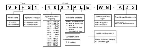
\* This code represents the factory default logic setting. You can switch from one input/output logic to the other using slide switch SW4. ⇒ See section 2.3.2.
