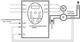
Feedback signals (1) DC: 4-20mA (2) DC: 0-10V
