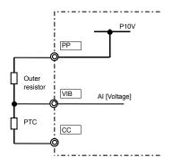
Connect the resistor rated 1/4 watts 3.3k ohm between terminal PP and VIB.
