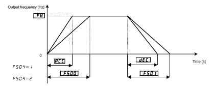
Acceleration/deceleration time 1 is initially set as the default. Acceleration/deceleration time 2 can be selected by changing the setting of the  $F S \mathcal{B} Y$ . Enabled if  $\mathcal{E} R \mathcal{B} d = I$  (panel input enabled)
