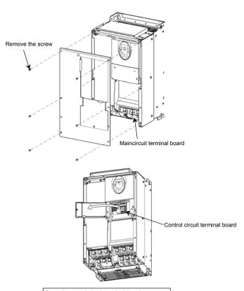
Open the control circuit terminal board cover.
