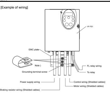
Note: Strip and earth the shielded cable, following the example shown in Fig.
