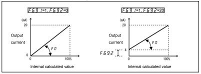
Note 1: When using the FM terminal for current output, be sure that the external load resistance is less than  $750\Omega$ . Note 2: Note that, if  $F \Pi S L$  is set to 7 (torque), data will be updated at intervals of more than 40 ms.
