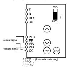
(11) Switching between analog setting and terminal setting from the operation panel
